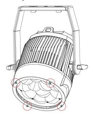
1. Remove the four (4) screws around the frame of the fixture's lens.
