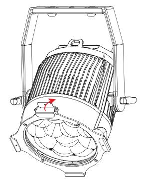
2. Align the gel frame holder on the frame, then re-install the four (4) screws to secure in place. Flip the latch open.
